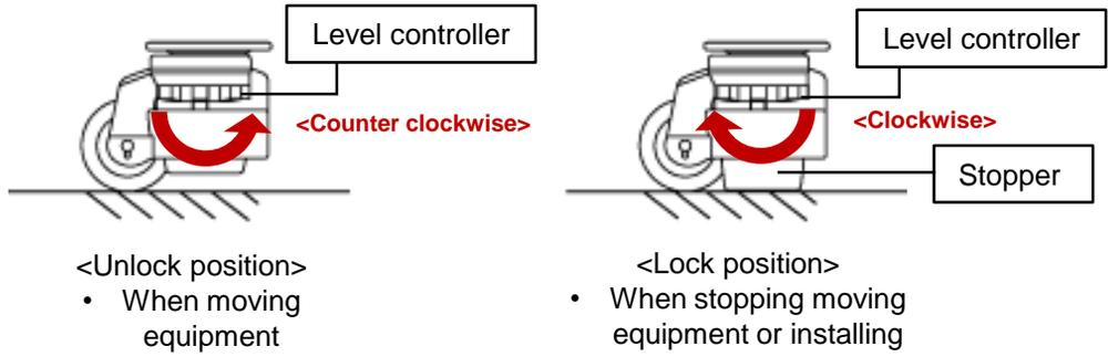
When installing equipment, fix the stopper to the floor by turning the level controller clockwise or counterclockwise.
