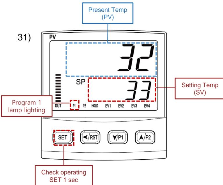
Out lamp is light is on and off during operating and heating.
