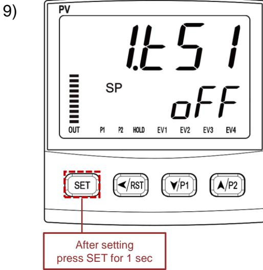
TS1(Time Signal) is setting for usage of function.
