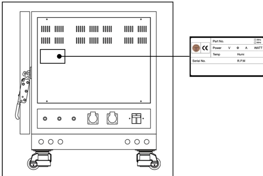
**!** Serial label shows the electric power specification of the unit.
